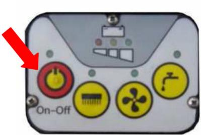
Press the brush button to activate suction and water delivery.
